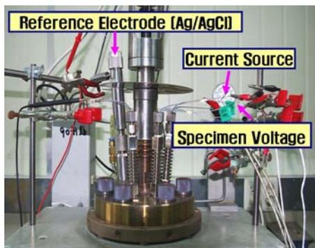
Fig. 1 Photo showing the upper head of an autoclave.
