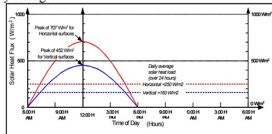
Figure 2. Variations of solar loads in the heat transfer analysis
