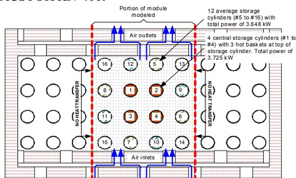
Figure 4. CATHENA Thermal-hydraulic Model
