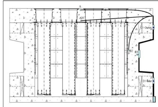
Figure 5. The location of installed thermocouples
