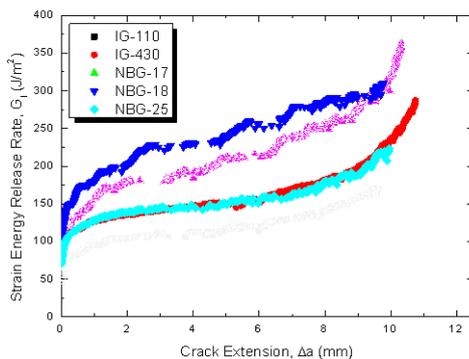
Fig. 3. Comparison of strain energy release rate-crack extension curves
