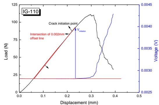
Fig. 1. Typical load-displacement curve for IG-110
