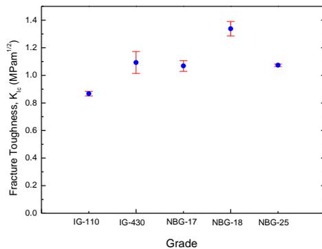
Fig. 2. Comparison of fracture toughness,  $K_{Ic}$
