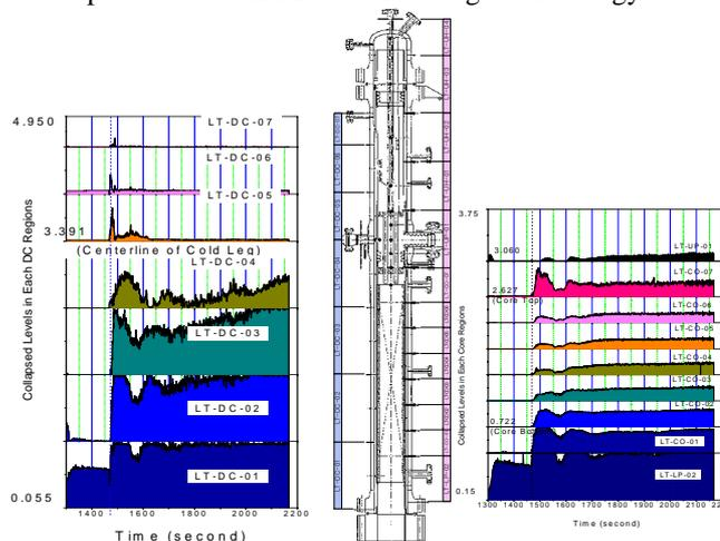
Fig. 2. Sectional water level variations in the downcomer and core regions during LB-CL-11
