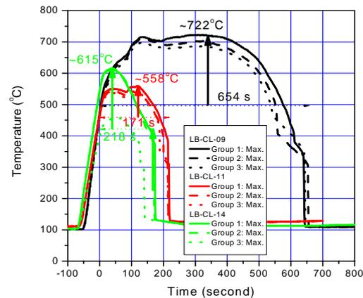
Fig. 1. Comparison of the maximum rod surface temperature between major Phase-2 tests
