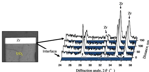
Figure 3. XRD Spectra for the Zry-4 cladding of a spent fuel of the average burn-up 41,000 MWd/tU.
