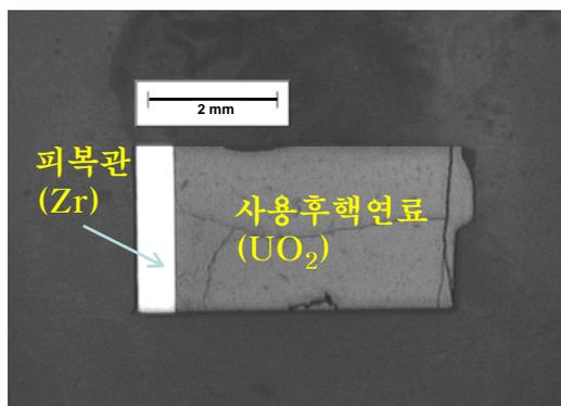
Figure 1. Spent fuel of average burn-up 41,000 MWd/tU discharged from Yeonggwang-2 nuclear reactor.
