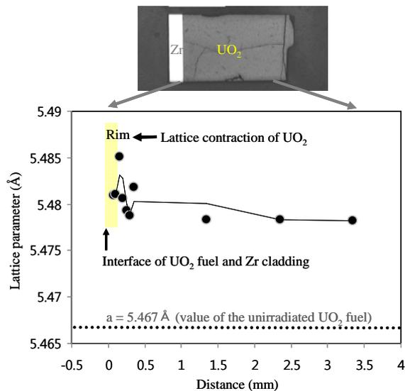
Figure 2. Changes in lattice parameter of  $\text{UO}_2$  (cubic) from a rim to the core of a spent fuel of average burn-up 41,000 MWd/tU discharged from Yeonggwang-2 nuclear reactor.
