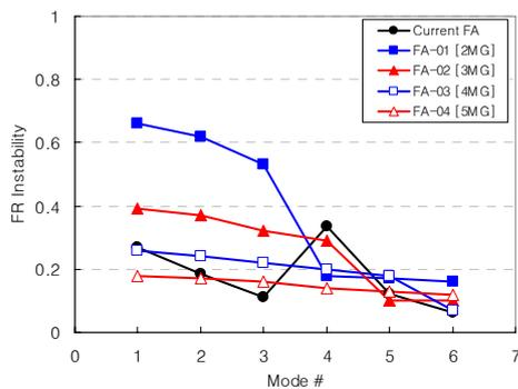
Fig. 5. FR Instability at BOL Hot Water Condition.
