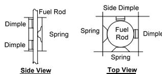
Fig. 2. FR connection with spring and dimple in grid cell
