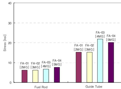
Fig. 6 Stress on FR and Guide Tube
