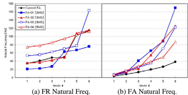
Fig. 4. FR and FA Modal Analysis (FR: BOL hot water condition, FA: cold air condition)
