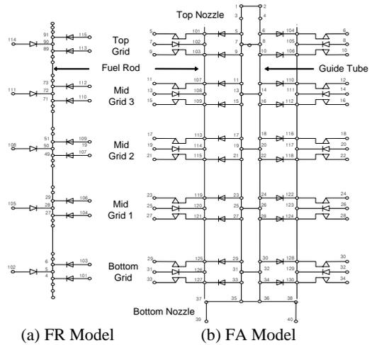
Fig. 3. Detail FR and FA Beam Model
