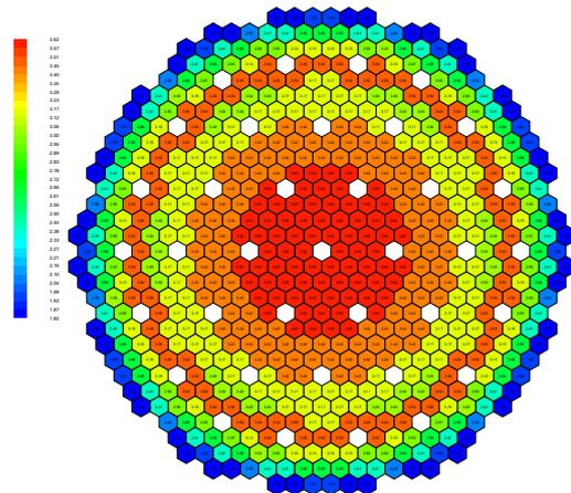
Figure 4 Core outlet coolant mean velocity distribution
