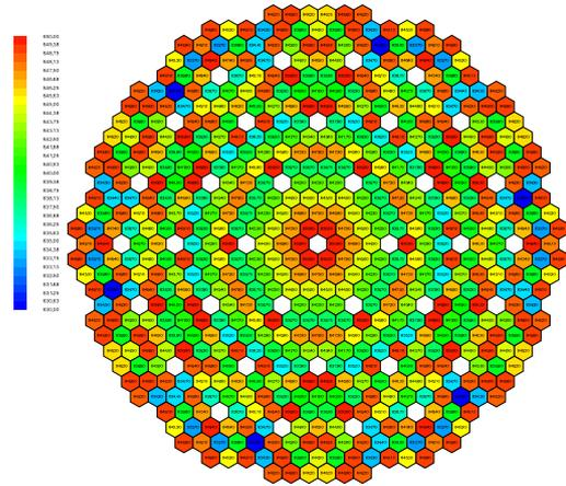
Figure 3 Maximum cladding mid-wall temperature with 2σ uncertainty distribution.
