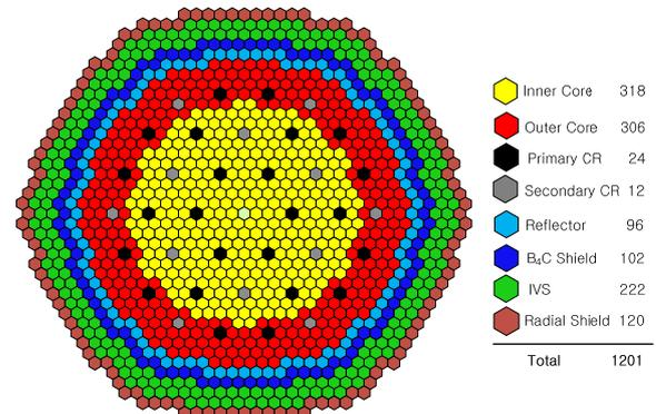
\* Another structural assembly instead of control rod was installed at the core centre
