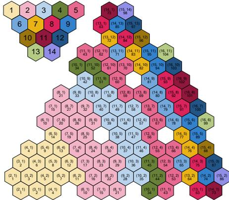
Figure 2 Assembly position and flow group of 1200 MWe SFR breakeven core
