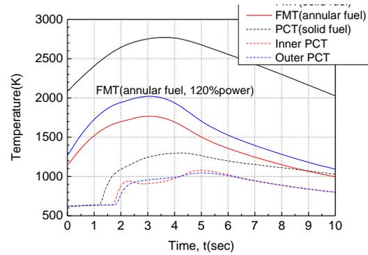
Fig. 5. Comparison of solid and annular fuel maximum and peak cladding temperatures during the REA.
