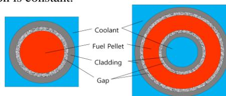
Fig. 1 Schematics of a solid fuel and a dual-cooled annular fuel.
