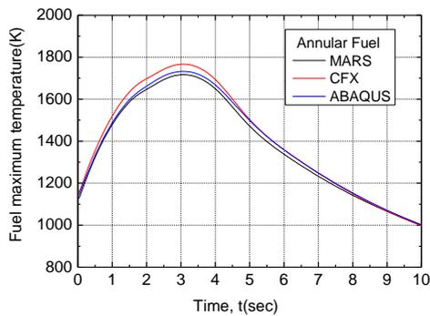
Fig. 2. Predictions of the annular fuel maximum temperature during the REA.
