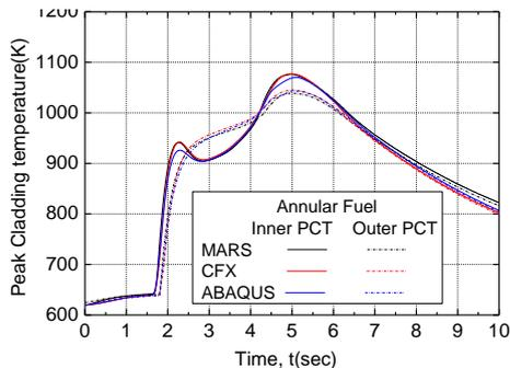
Fig. 3. Predictions of the annular fuel peak cladding temperature during the REA.
