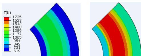
Fig. 4. Temperature contours of the annular fuel before and after the REA, i.e.,  $t=0$  sec and  $t=3.1$  sec.
