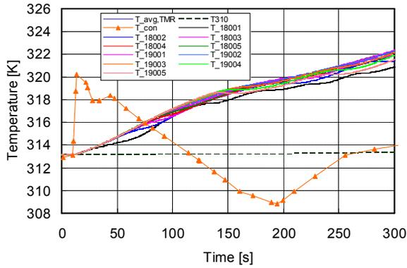
Fig. 2. Temperature transients of transmitter and transmitter room for 2.5% ROH break
