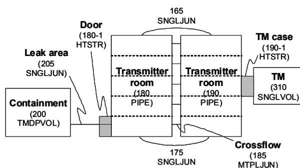
Fig. 1. Nodalization diagram of transmitter and transmitter room for the analysis with MARS.
