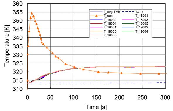
Fig. 4. Temperature transients of transmitter and transmitter room for 100% ROH break
