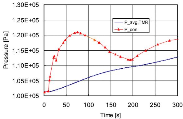
Fig. 3. Pressure transients of transmitter and transmitter room for 2.5% ROH break
