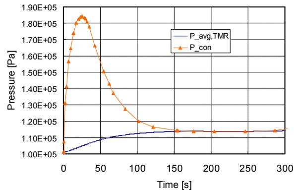
Fig. 5. Pressure transients of transmitter and transmitter room for 100% ROH break
