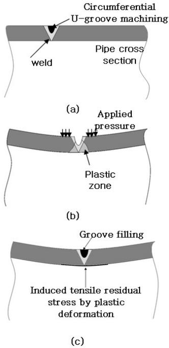
Fig. 2 Suggested new method process for mitigating tensile residual stresses induced on the inside wall of dissimilar metal butt welded pipes.
