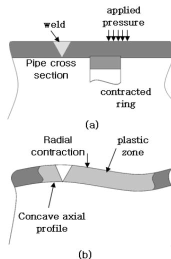
Fig. 1 Schematic drawing of step (a) and (b) for Mechanical Stress Improvement Process (MSIP).
