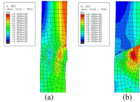
Fig. 3 Calculated final residual stress distribution obtained from modeling of new method process. (a) is the axial residual stress distribution and (b) is the hoop residual stress distribution.
