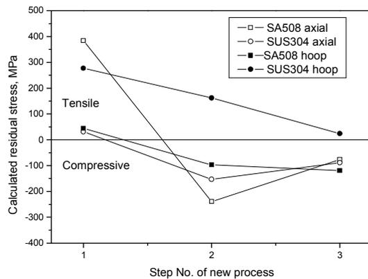
Fig. 4 Variation of calculated residual stresses near root region on each step of the new method (1: initial state, 2: after pressing step, 3: final step).
