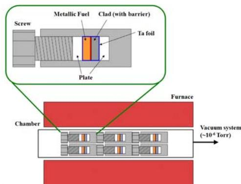
Fig. 1. Schematic illustration of diffusion couple test between metallic fuel and clad
