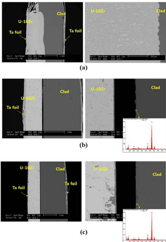
Fig. 3. Low magnification cross-sectional SEM results of interface structures of the specimens after the diffusion couple test (a) without diffusion barrier and ZON film with hydrogen flow rate of (b) 30 sccm and (c) with 50 sccm.
