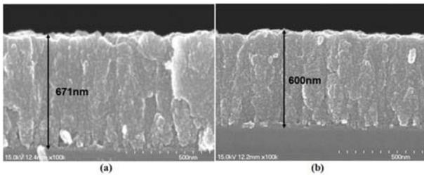
Fig. 2. cross-sectional view of as deposited ZON thin films with hydrogen flow rate of (a) 30 sccm and (b) with 50 sccm.
