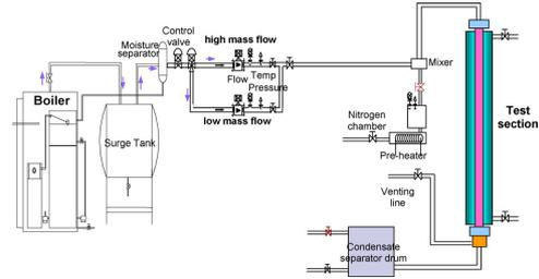
Figure 1. Schematic Drawing for Experiment
