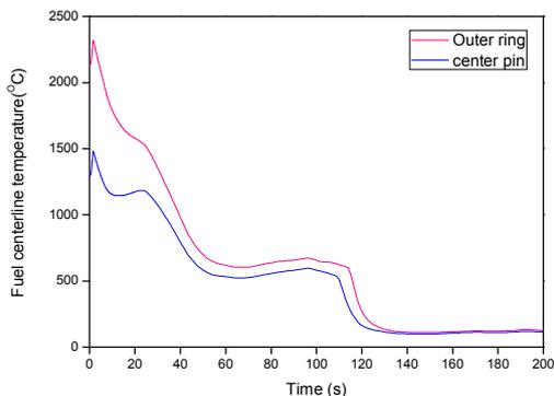
Figure 4 Fuel centerline temperature
