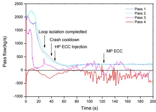
Figure 2 Circuit flow and ECC signal
