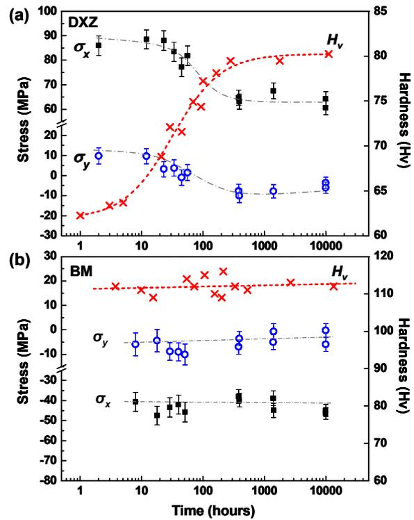
Fig. 2. Time-dependent residual stresses ( $\sigma_x$ ,  $\sigma_y$ ) measured at (a) DXZ (average within  $\pm 5$  mm) and (b) BM (base material, average of 30 and 50 mm). Calculated volume fraction ( $f_r$ ) of precipitates (dotted profile) is superimposed on the measured hardness (cross marks).
