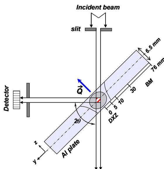
Fig. 1. Schematic of the experimental setup for the neutron diffraction measurements (DXZ: dynamic recrystallized zone, BM: base material).
