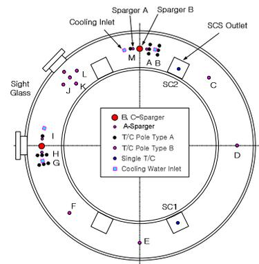
Fig. 2. Locations of the Thermocouple (T/C) Poles
