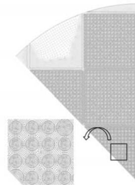
Fig. 2. Mesh generation for 1/8 section of TN24P cask.
