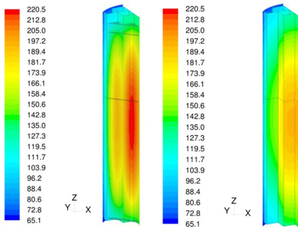
Fig. 3. Temperature distribution in spent fuel assemblies (left) and basket (right).
