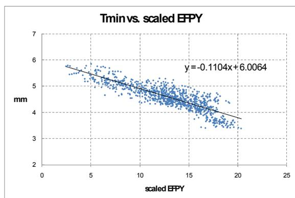
Figure 2 Minimum wall thickness vs. scaled EPFY
