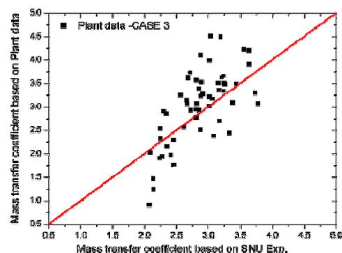
Figure 1 Mass Transfer Coefficients calculated from plant data and plaster of Paris
