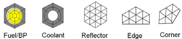
Fig. 2. Basic unit cells used in the present model.
