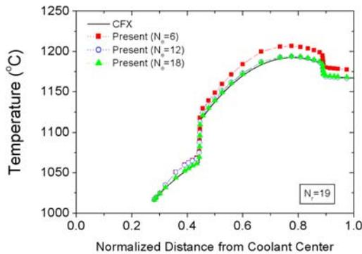
Fig. 5. Comparison of the predicted temperature profiles in the seven unit cells.
