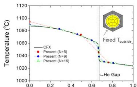
Fig. 3. Comparison of the predicted temperature profiles inside the single unit cell containing fuel compact.
