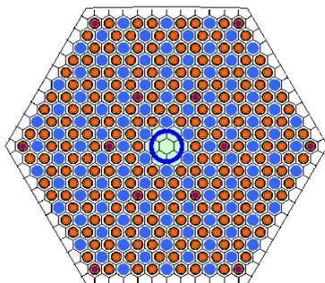
Fig. 1. A typical arrangement of unit cells in a prismatic fuel block.
