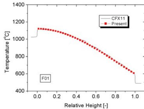
Fig. 6. Comparison of the predicted axial temperature profiles along the center of the selected fuel compact.
