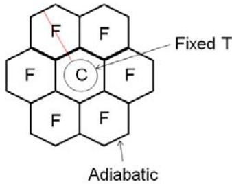
Fig. 4. A layout of seven unit cells and boundary conditions.
