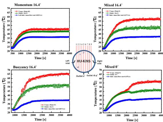
Fig. 5. Temperature pattern of outlet part and maximum temperature point in the passage of time
