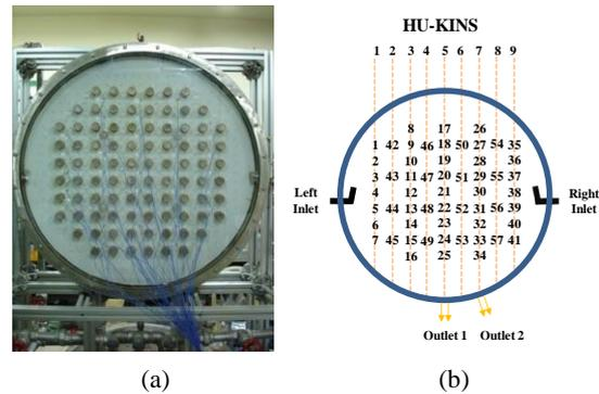
Fig. 2. (a) Thermocouples inserted into the HUKINS, (b) monitoring positions
