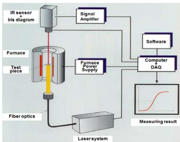
Fig 4. Schematic Diagram of LFA 427
