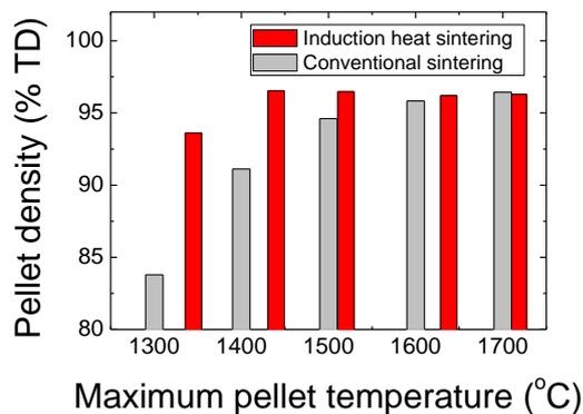
Fig. 2. Density of sintered  $UO_2$  pellets as a function of the sintering temperature.
