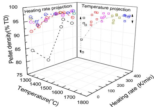
Fig. 4. Densities of sintered  $UO_2$  pellets as a function of the heating rate and sintering temperature.
