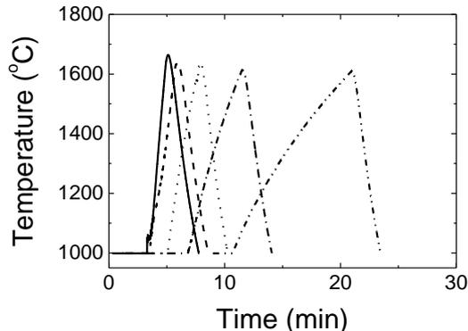
Fig. 3. Typical heating curves for selected sample pellets adapting different heating rates.
