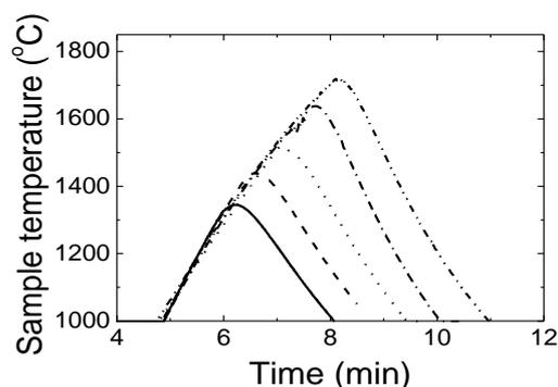
Fig. 1. Time-temperature graphs showing a temperature increase of UO<sub>2</sub> pellets
