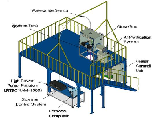
Figure 6. Experimental facility for the performance test in sodium
