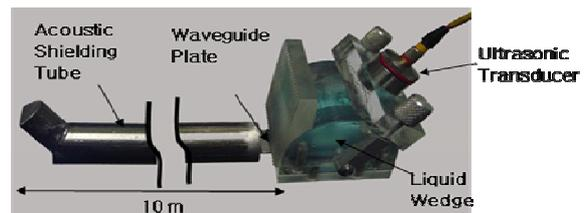
Figure 2. Waveguide sensor modules
