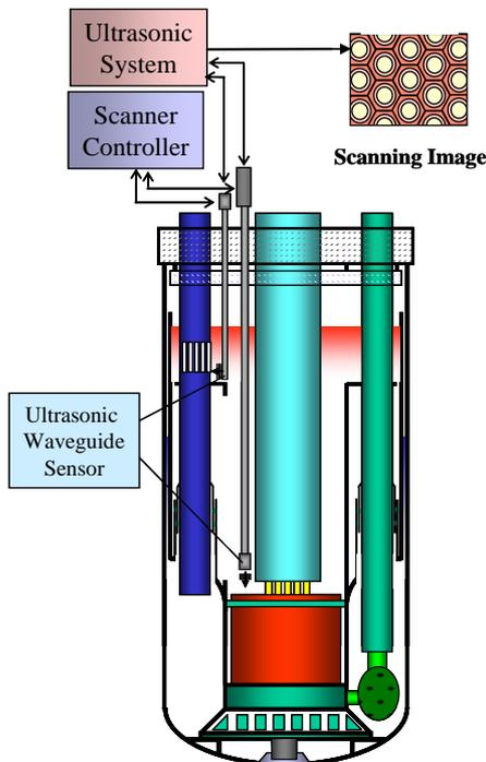
Figure 1. Under-sodium visual inspection of reactor internals using ultrasonic waveguide sensor
