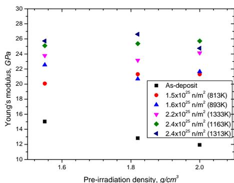
Fig. 2. Variation of the Young's modulus of PyC layer deposited from methane as a function of pre-irradiation density in different neutron irradiation conditions.
