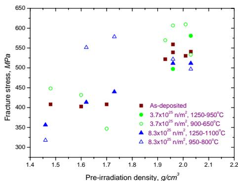
Fig. 3. Variation of the fracture stress of PyC layer deposited from propane as a function of pre-irradiation density in different neutron irradiation conditions.
