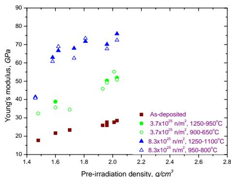
Fig. 1. Variation of the Young's modulus of PyC layer deposited from propane as a function of pre-irradiation density in different neutron irradiation conditions.
