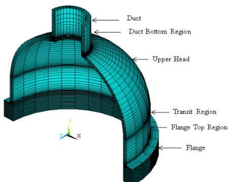
Fig. 1 Finite element model of the reactor vessel head with elevated temperature
