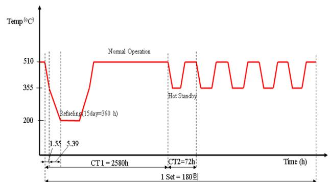
Fig.3 Coolant temperature distribution for two cycle types
