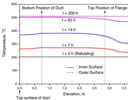
Fig. 5 Temperature distributions along elevations during the heat-up operation of cycle type-1
