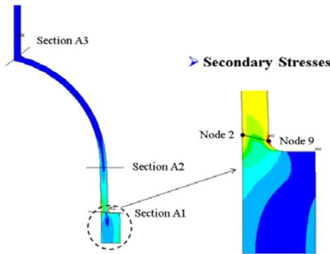
Fig. 4 Evaluation cross sections of a reactor vessel head
