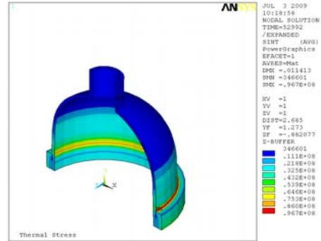
Fig. 6 Linearized stresses in A1 section for cooldown (Minimum stress time point)
