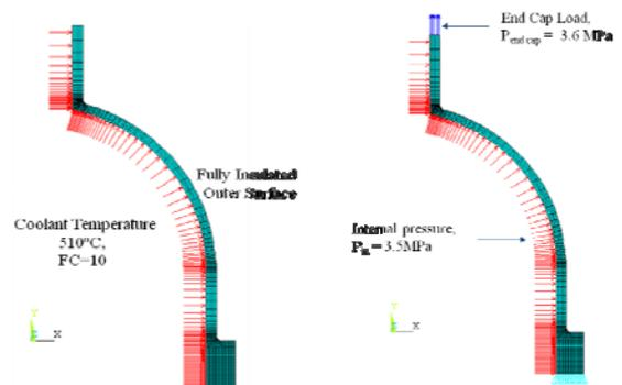
Fig. 2 Thermal and mechanical boundary conditions for a reactor vessel head
