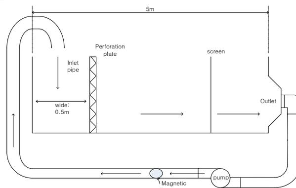
Fig. 1. Schematic of Flume Assembly
