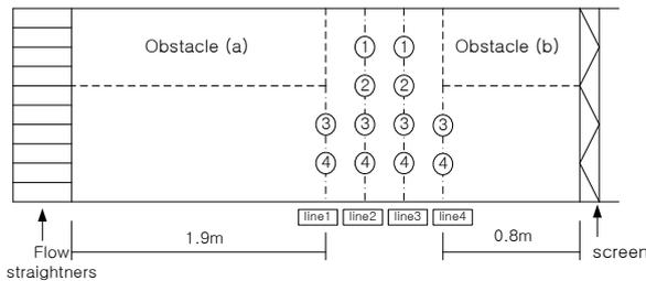
Fig. 3. Schematic of Flume Assembly
