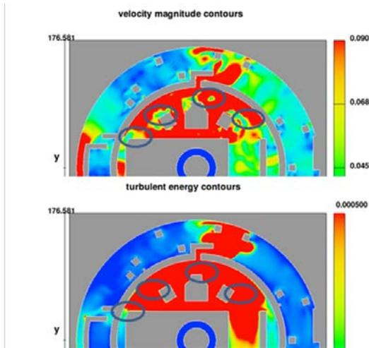
Fig. 2. Compare of tumbling velocity and turbulence kinetic energy on OPR1000 floor at 26.85m
