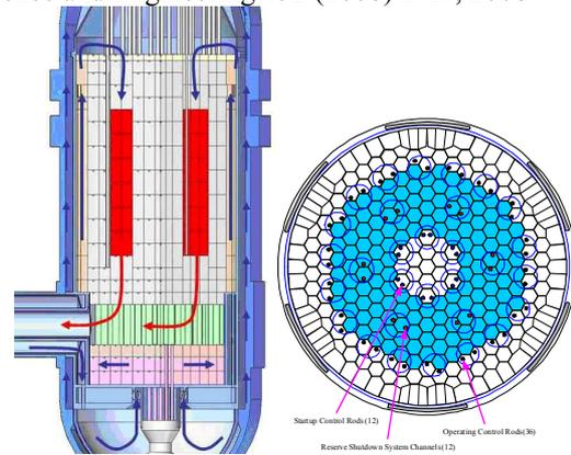
Fig. 1 DB-MHR Core Design Configuration
