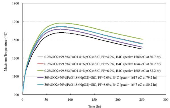
Fig. 4 Peak Fuel Temperature Transients during LPCC
