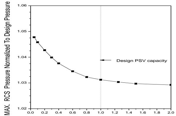
Fig. 3. RCS pressure behavior during loss of load
