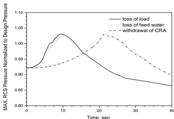
Fig. 1. RCS pressure behavior during various transients.
