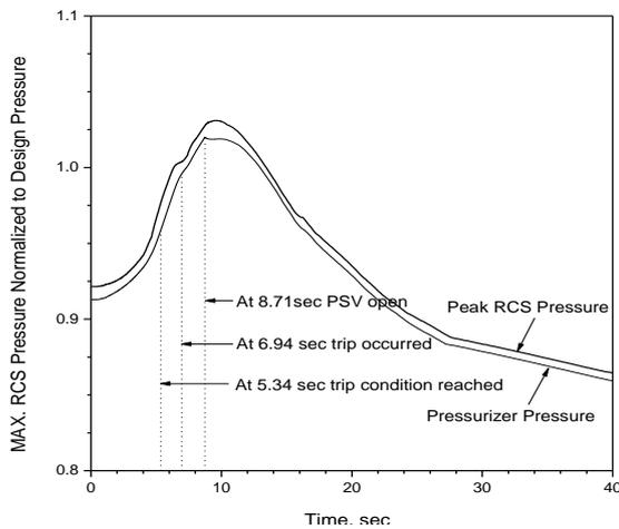
Fig. 2. RCS pressure behavior during loss of load
