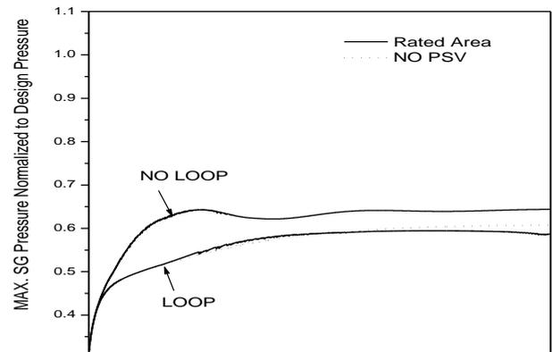
Fig. 4. SG secondary pressure behavior during loss of load
