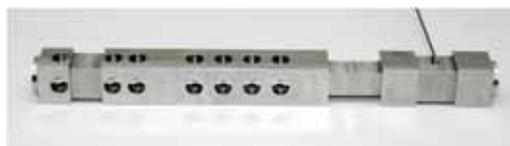
Fig. 2. 1/5-scale core simulator
