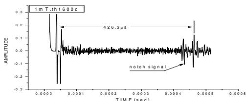
Fig. 2. Delay time at a 1600°C Temperature (Sensor length : 1000mm)
