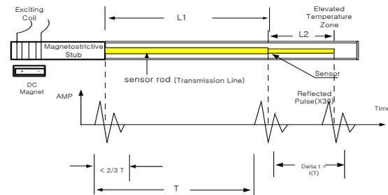
Fig. 1. Ultrasonic Thermometer using the Pulse-Echo Method
