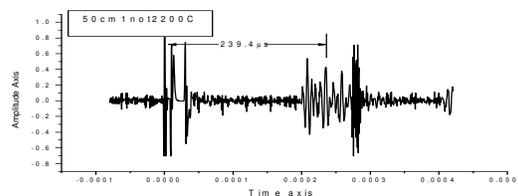
Fig. 3. Delay time at a 2200°C Temperature (Sensor length : 500mm)
