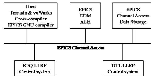
Figure 1. Integrated development environment and distributed control system
