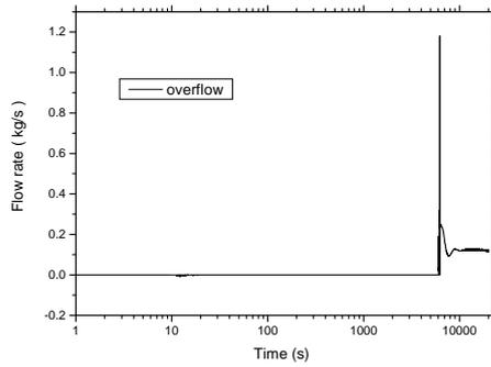
Fig.2. DHX over-flow to PDRC system at LOF
