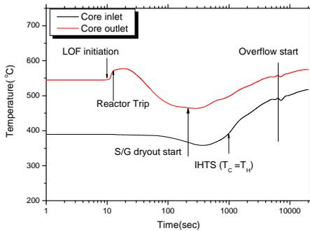
Fig.4. Coolant temperatures behaviors at Core inlet/outlet
