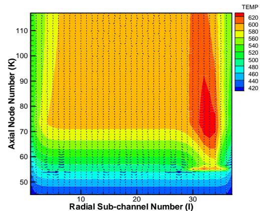
Fig. 7 Temp. and flow profiles for the 24 edge blockage
