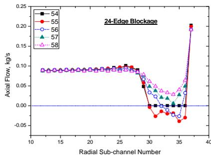
Fig. 5 Axial flow distribution for the 24-edge blockage
