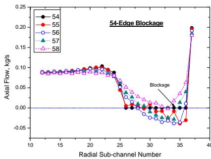
Fig. 4 Axial flow distribution for the 54-edge blockage
