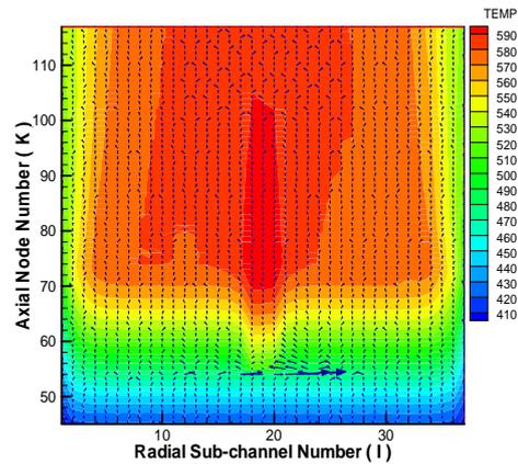
Fig. 2 Temp. and flow profiles for the 6-central blockage
