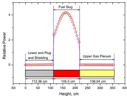
Fig. 1 Axial power distribution for MATRA inputs
