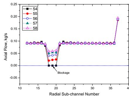
Fig. 4 Axial flow distribution for the 6-central blockage
