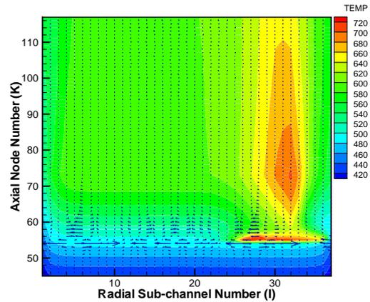
Fig. 6 Temp. and flow profiles for the 54 edge blockage
