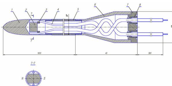
Fig. 5. Drawing of local velocity transducer.
