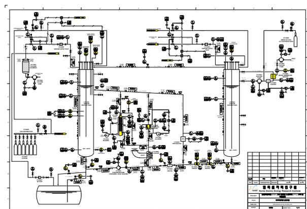
Fig. 3. P&ID of sodium loop for testing and calibration of manufactured transducers.
