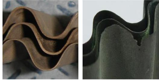
Figure 3. A cross sectional observation of as-received and the SiC coated Hastelloy X sheets shaped for the decomposed sulfuric acid channel before and after immersing in 98% H<sub>2</sub>SO<sub>4</sub> for 80 hrs (a) and 348hrs (b) at 300 °C.
