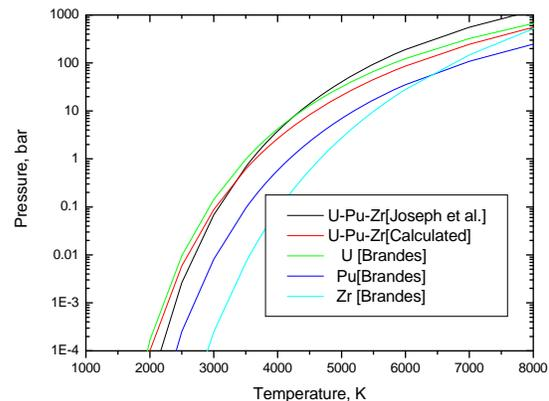
Fig.1. Relationship of vapor pressure and temperature of U-Pu-Zr fuel alloy and each element
