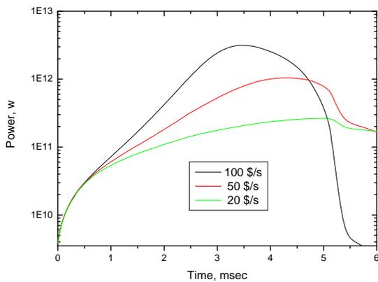
Fig.2. Power change during the power excursion of various reactivity insertion rates
