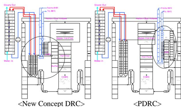
Figure 1. MARS-LMR nodalization for KALIMER 600 MWe
