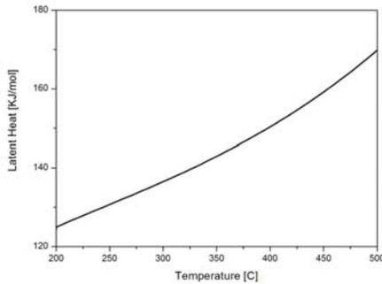
Fig. 2. Latent Heat of  $H_2SO_4$  Decomposer
