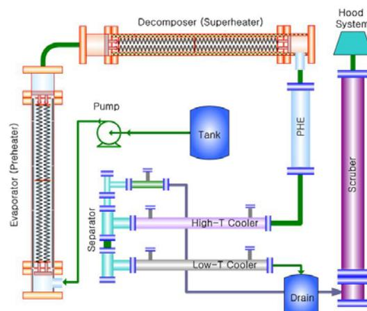
Fig. 1. Schematic Diagram of a Sulfuric Acid Loop
