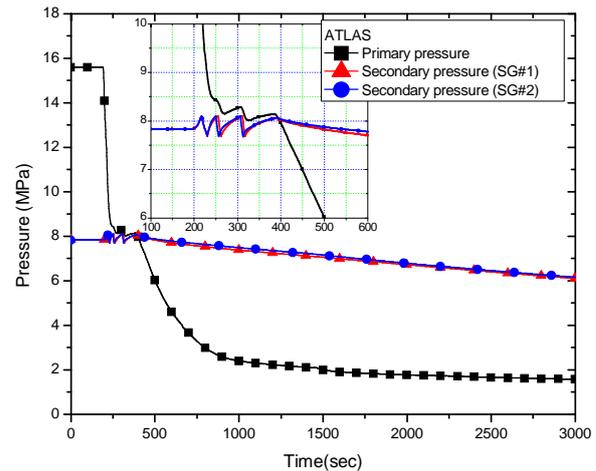
Fig. 1 Measured primary and secondary pressure
