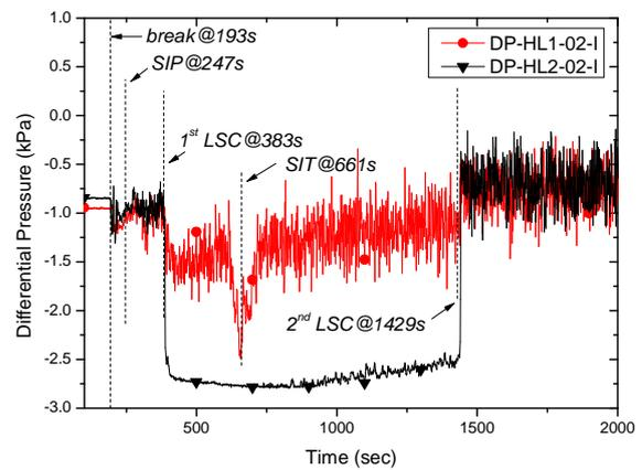
Fig. 4 Differential pressures in the hot leg 1 and 2
