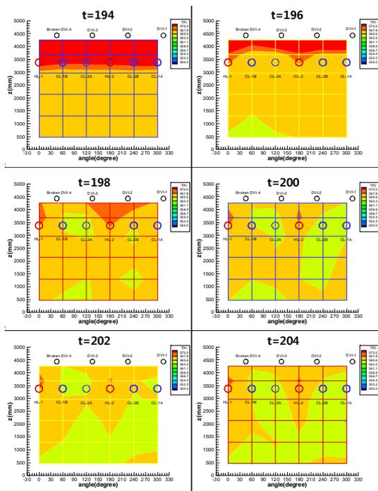
Fig. 3 Fluid temperature contour in the down-comer
