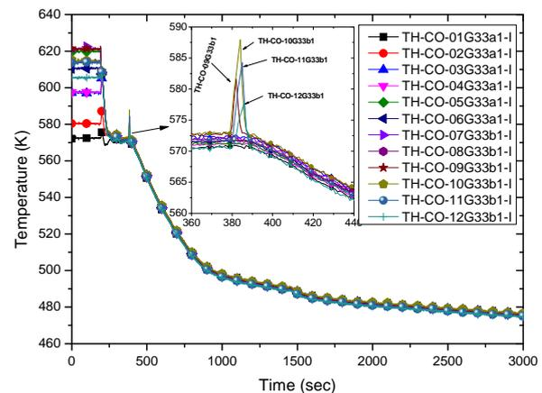
Fig. 2 Measured PCT of the heaters in G33a1 and G33b1
