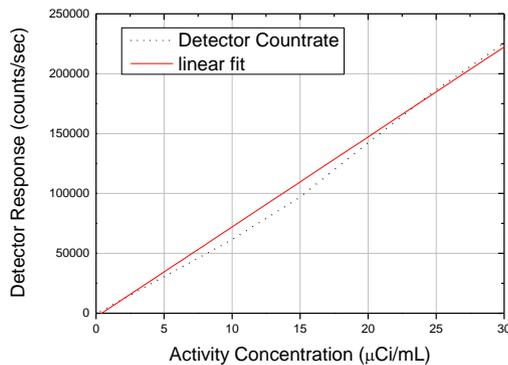
Fig 4. Linearity characteristics on Blood activity measurement system. The solid line represents a linear fit to countrate from 0.1  $\mu\text{Ci/mL}$  to 30  $\mu\text{Ci/mL}$ .
