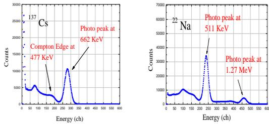
Fig 3. Pulse Height Spectra of Co-60, Cs-137, Na-22, F-18 sources obtained with detector of GSO for energy resolutions
