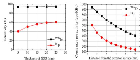
Fig 2. (a) Sensitivity as a function of GSO thickness, (b) Count rates as a function of the distance from the detector surface.
