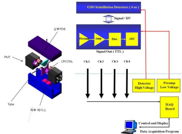
Fig. 1. A Schematic of the Blood Activity Measurement System.
