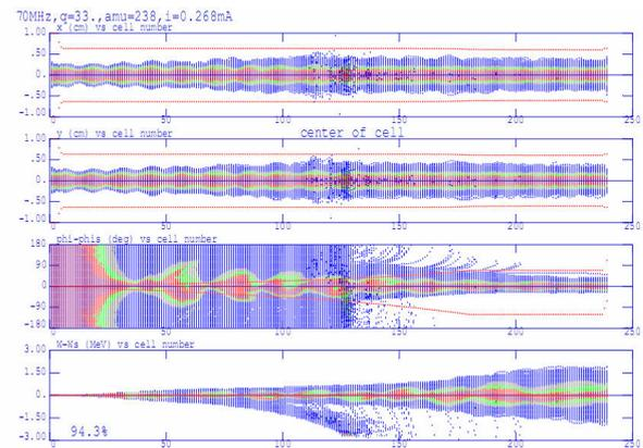
Fig. 2. Uranium Beam Traces along Heavy Ion RFQ
