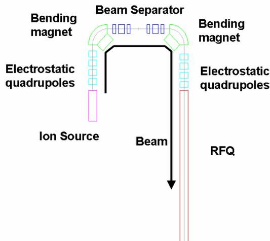
Fig. 1. LEBT to match  $^{238}\text{U}^{32+}$ ,  $^{238}\text{U}^{33+}$  and  $^{238}\text{U}^{34+}$  from an ion source to a RFQ
