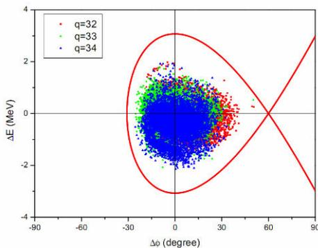
Fig. 4. RF bucket with the three charge states
