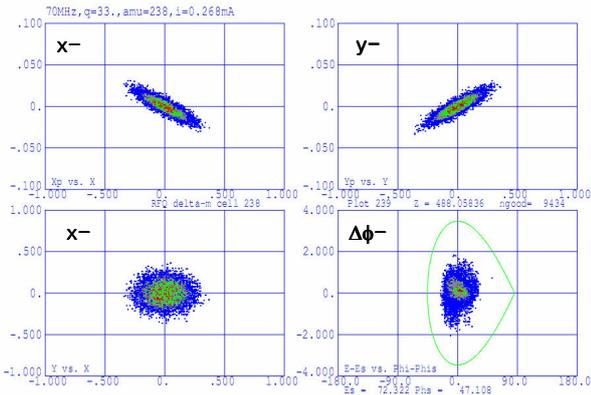
Fig. 3. RFQ Output Uranium Beam in Phase Space
