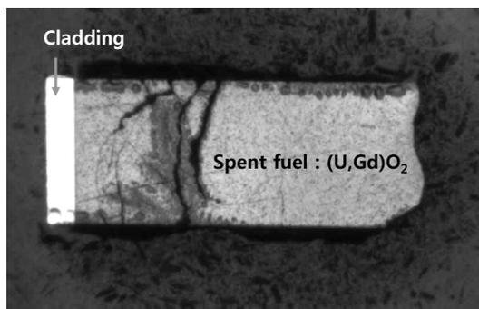
Figure 1. Prepared spent (U,Gd)O<sub>2</sub> fuel specimen.
