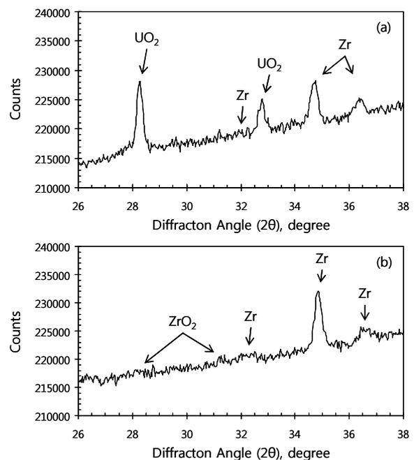
Figure 2. XRD Spectrum of a zirlo cladding: (a) the inner layer, (b) the outer layer.
