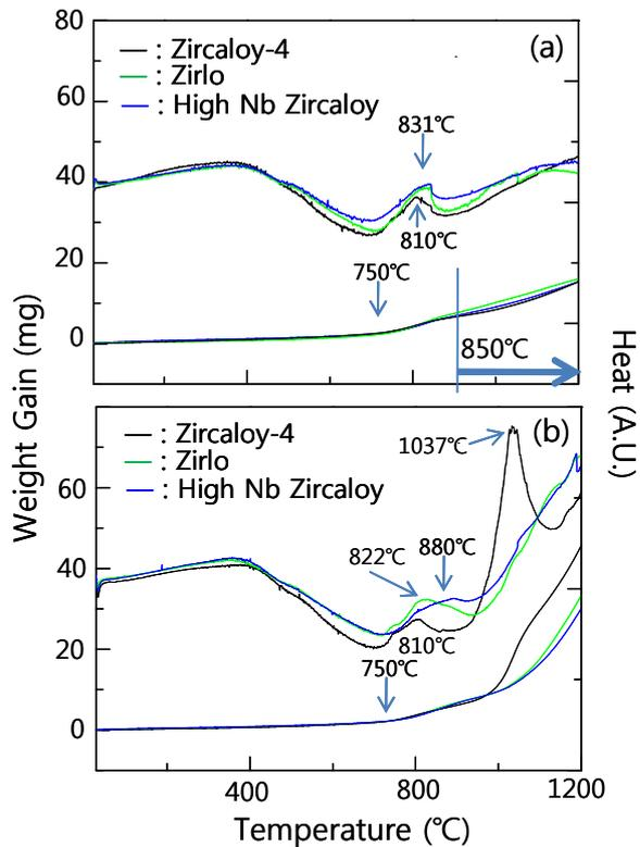
Figure 3. TG-DTA curves for the Zircaloy oxidation under oxygen. [stay 5 hours at 850°C (a); continue to 1200°C (b)]
