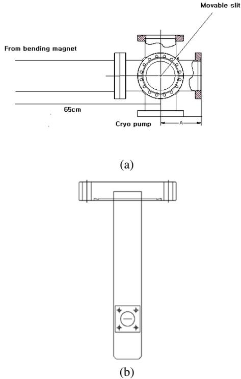
Figure 3: (a) Energy spread measurement chamber; (b) The slit plate and its holder. The slit width is 0.01mm.
