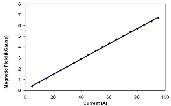
Figure 2: Magnetic field of the bending magnet
