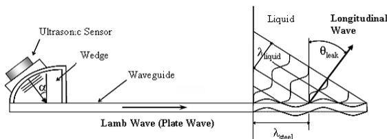
Fig. 1. Ultrasonic waveguide sensor.
