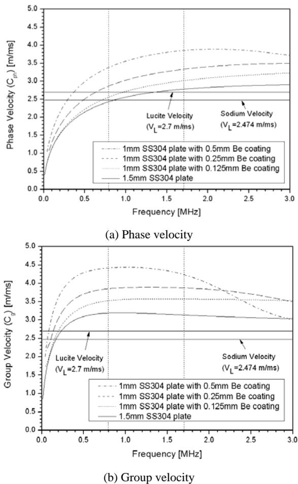
Fig. 3. Dispersion curves of the  $A_0$ -mode Lamb wave of Be-coated SS304 plates in ultrasonic waveguide sensor.
