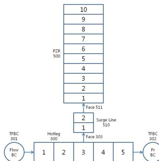
Fig. 1. Nodding diagram of simple in-surge pressurizer.
