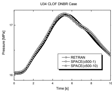
Fig. 2. Calculation results of RETRAN and SPACE code.
