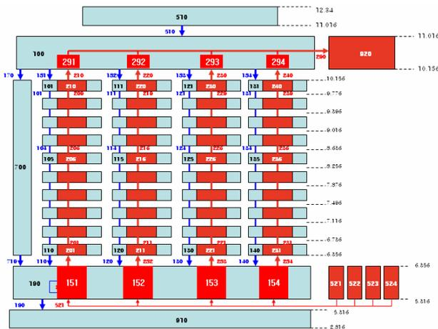
Figure 1 Nodalization of SMART system for simulating the steady state condition
