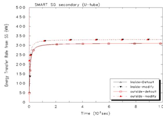
Figure 2 Predicted thermal power of SMART
