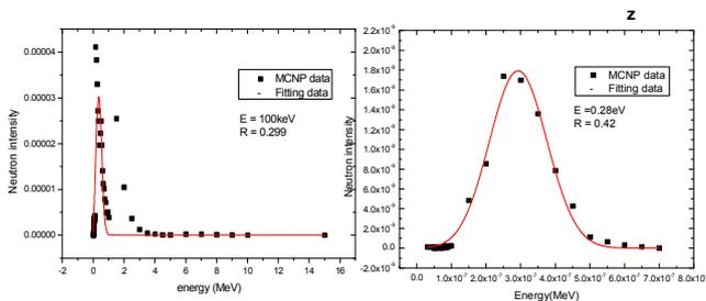
Fig. 1. Neutron energy resolution in the slowing down medium.
