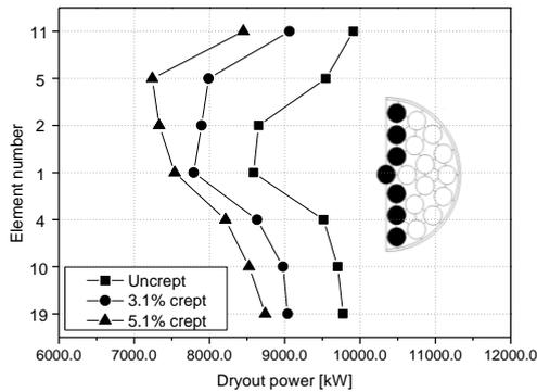
Fig.3 Dryout power distribution at central-positioned elements.
