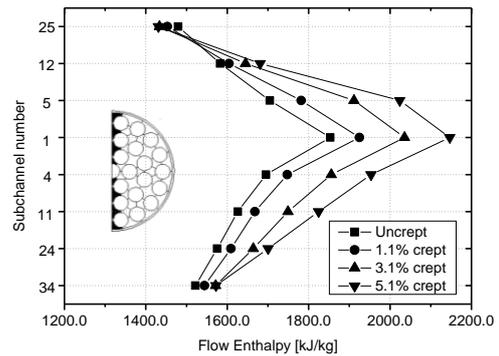
Fig.4 Flow enthalpy at central-positioned subchannels.
