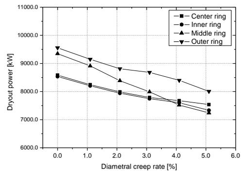
Fig.2 Dryout power at each ring with creep rate
