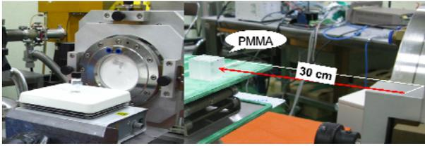
Fig. 1. 45 MeV beam line of MC-50 cyclotron at KIRAMS.
