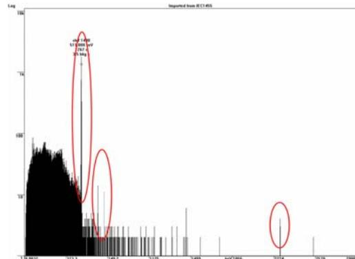
Fig. 4 Gamma-ray spectrum of PMMA (the first circle is 511 keV, the second is  $^{10}\text{C}$  (715 keV), and the last is  $^{14}\text{O}$  (2312 keV)).
