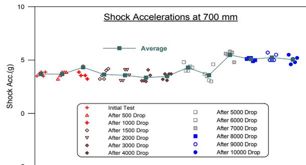
Fig.8 Drop impact at 700mm for improved CRDM
