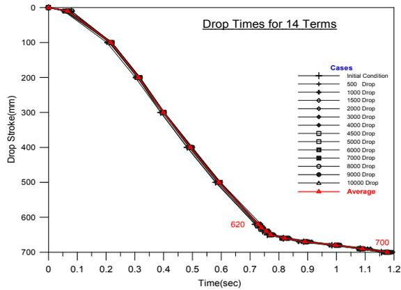
Fig.3 Drop curve for improved CRDM
