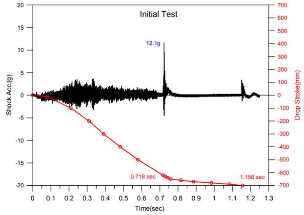
Fig.5 Drop impact at the first drop for improved CRDM
