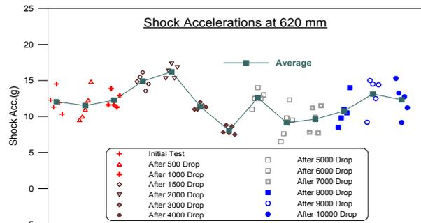
Fig.7 Drop impact at 620mm for improved CRDM
