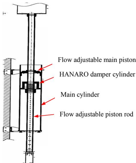
Fig. 1 Improved CRDM damping mechanism
