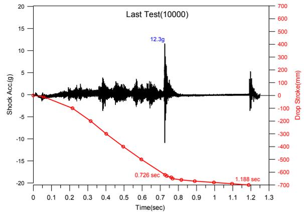
Fig.6 Drop impact at the last drop for improved CRDM
