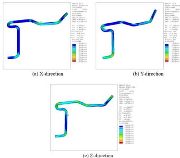
Fig. 4. Stress intensity distribution of NISO model by the mode combination
